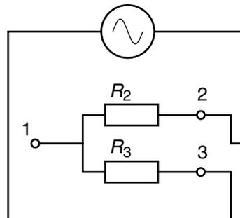
$$b) R_{eq.} = \frac{R_2 \cdot R_3}{R_2 + R_3} = 720 \Omega$$
