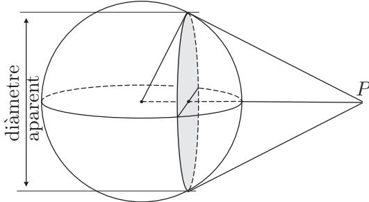
$$\begin{aligned} d &= 2 \cdot 6371 \cos \alpha = 2 \cdot 6371 \sqrt{1 - \sin^2 \alpha} \\ &= 2 \cdot 6371 \sqrt{1 - \left(\frac{6371}{6371 + 8000}\right)^2} = [11421.44 \text{ km}]. \end{aligned}$$
