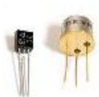
A solid semiconductor device used to amplify and switch electronic signals.
