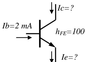
$$I_c = h_{FE} \cdot I_b = 100 \cdot 2\text{mA} = 200\text{ mA} = 0.2\text{ A}$$
