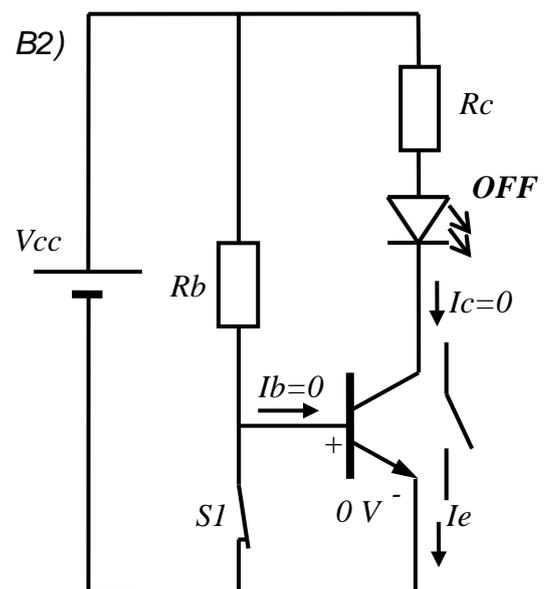
Circuit \_\_\_\_\_: When the switch is ON a current passes through the resistor into the base of the transistor. Then the transistor allows collector current to flow and the LED comes on.
