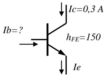
**12c** As with diodes, a voltage of  $0.7\text{V}$  is necessary across the base-emitter to activate the transistor. In this circuit you can see the formula to calculate the current into the base. Then you can calculate the current into the collector.
