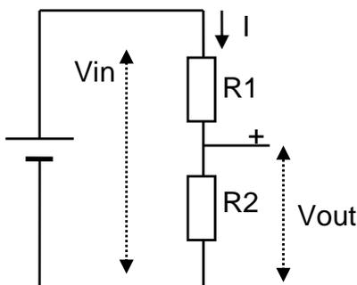
$$V_{out} = V_{in} \cdot \frac{R_2}{R_1 + R_2}$$
