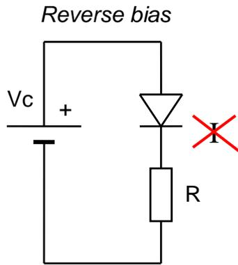
A diode is a semiconductor device that allows current to flow in one direction. It can be used for protection, to block signals, to change AC to DC, etc.
