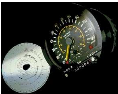
A typical tachometer and chart used in most commercial vehicles. A school minibus may be fitted with this device - particularly if the minibus is used on European roads where the device is required.
