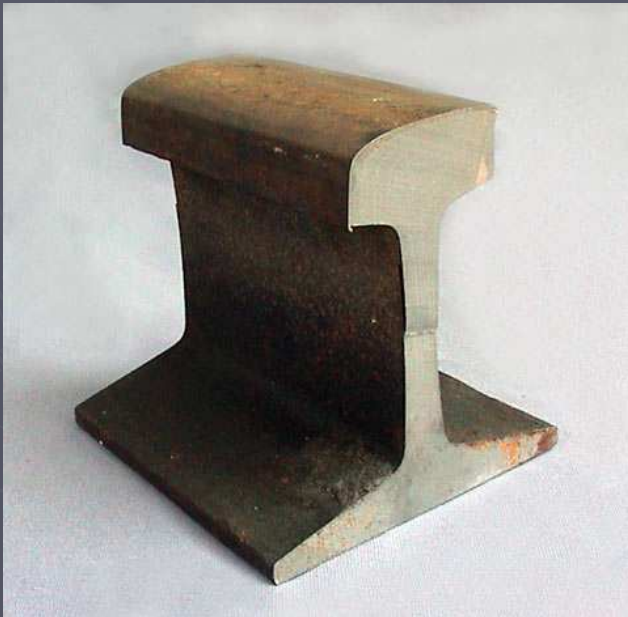
Profile of a railway track and other common sections
