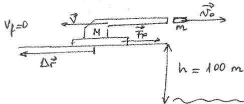
$M = 5000 \text{ kg} ; m = 40 \text{ kg} ; v_0 = 200 \frac{\text{m}}{\text{s}}$
