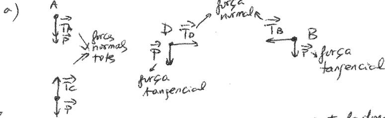
b)  $T_A + P = m \frac{v_A^2}{l}$  ;  $T_A = m \left( \frac{v_A^2}{l} - g \right)$
