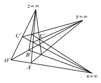
FIGURE 11. A projective frame  $\{O', A', B', C', U'\}$  is defined by one point more than an affine frame  $\{O', A', B', C'\}$ . The unit point U' is additionally taken although any other point suffices. Line coordinates are not parallel in general but they are concurrent at points having the corresponding coordinate equal to infinity.
