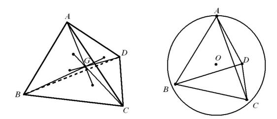
FIGURE 9. The centroid G is the intersection of the medians. The circumcentre O is the centre of the sphere circumscribed to the tetrahedron.
