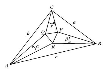
FIGURE 3. Morley's theorem. The intersections of the trisectors of the interior angles form an equilateral triangle.
