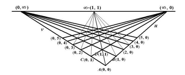
FIGURE 12. Example of a projective grid in the plane. The projective frame is  $\{A, B, C, D\}$  where D is the unit point. Four points, no three of which are collinear, define a projective grid if we assign coordinates to them. Points with integer values of coordinates are displayed. The line joining points at infinity is called the line at infinity.
