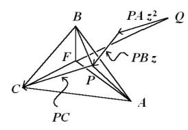
FIGURE 2. The addition of distances from any point *P* to the three vertices is minimal when *P* is the Fermat point *F* provided that the three interior angles are lower than  $2\pi/3$ .
