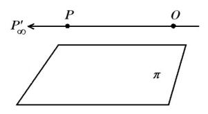
FIGURE 9. Projection yielding a point at infinity.
