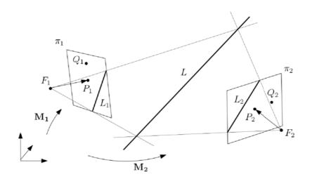
FIGURE 2. A line symmetry projected to two cameras
