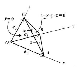
FIGURE 1. Affine frame defining, in the geometric space E, a coordinate system with origin in O and vector basis  $\{e_1, e_2, e_3\}$ .  $\{O, A, B, C\}$  is a basis for points,  $\{OA, OB, OC, AB, AC, BC\}$  is a basis for lines, and  $\{OAB, OAC, OBC, ABC\}$ , whose equations are indicated, is a basis for planes and dual space  $E^*$ .
